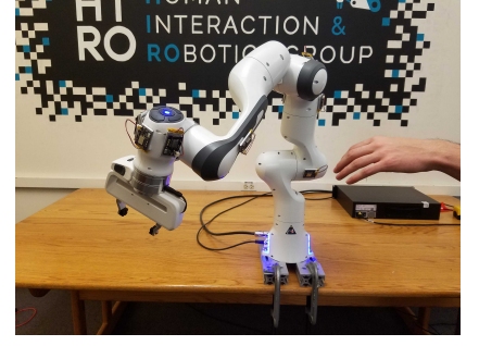
(c) Post-Contact: After the external force threshold exceeded, a reactive behavior moves the robot in the direction and magnitude of the applied force.
